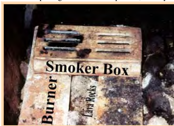
Picture of the Smoker Box sitting perpendicular to the gas burners.
